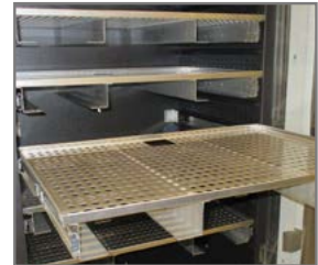
Telescopic rails for easier loading of the chamber
