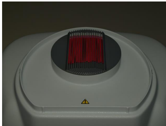
Figure 41: 0.25ml IMV straws positioned on H01 head
