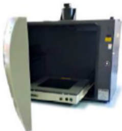
Attach the camera, slide the transilluminator into place, and put on the camera cover
