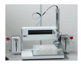
Applications: Waste oil, Transformer oil, Engine oils, Hydraulic fluids ASTM D663, D974, ISO 3771, IP400
